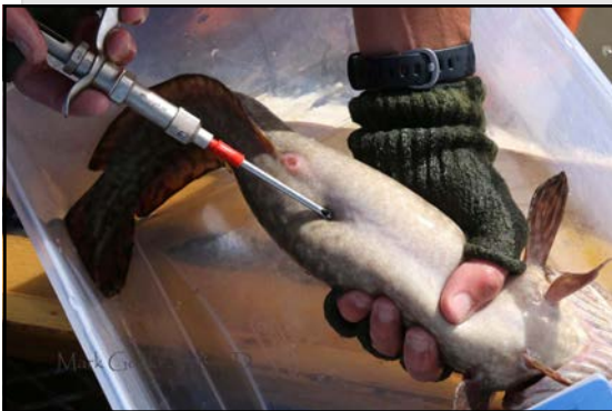
A tiny PIT tag is inserted into the belly of a burbot. (Right) A PIT antennae installed on the Green River to record when tagged fish move upstream.
