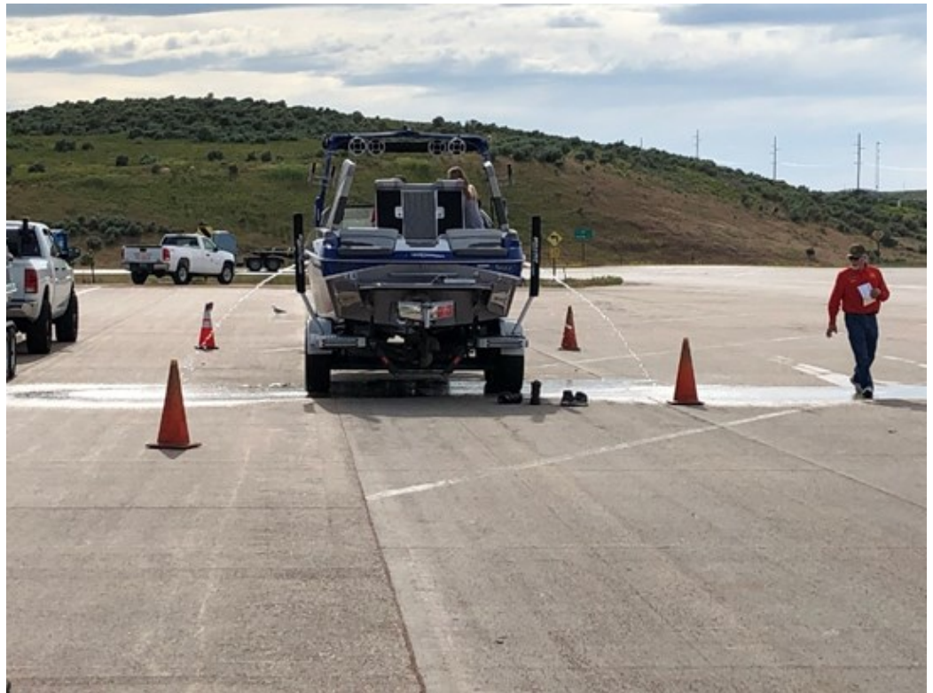
Example of a boat the owner who thought the boat was dry, but it wasn't. Boat discharging over 5 gallons of water from its ballast tanks.
