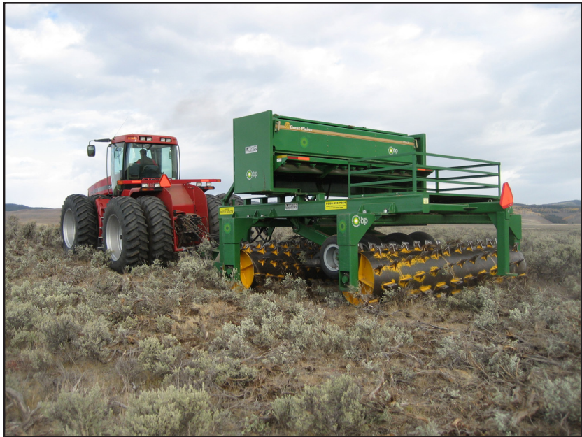
Figure 38. Lawson aerator provides mechanical disturbance with the option of incorporating seed into the treatment based on-site specific objectives
