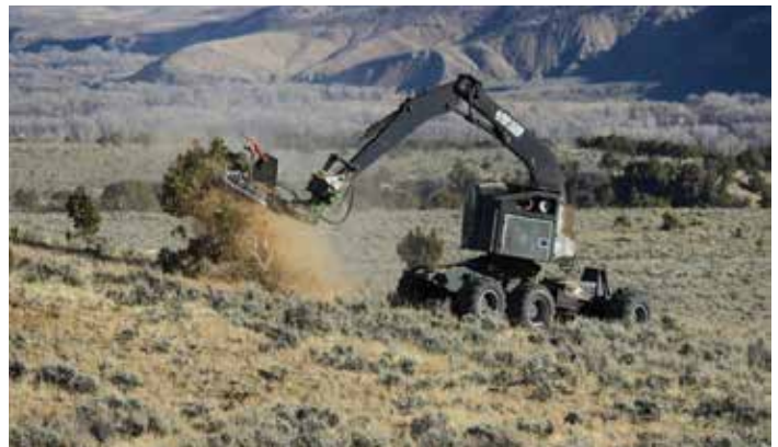
Heavy Equipment grinding a juniper near Savery.
