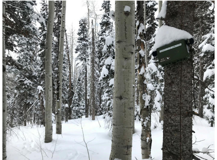
Autonomous Recording Unit (ARU) deployed during early-season surveys to record American Goshawk calls.
