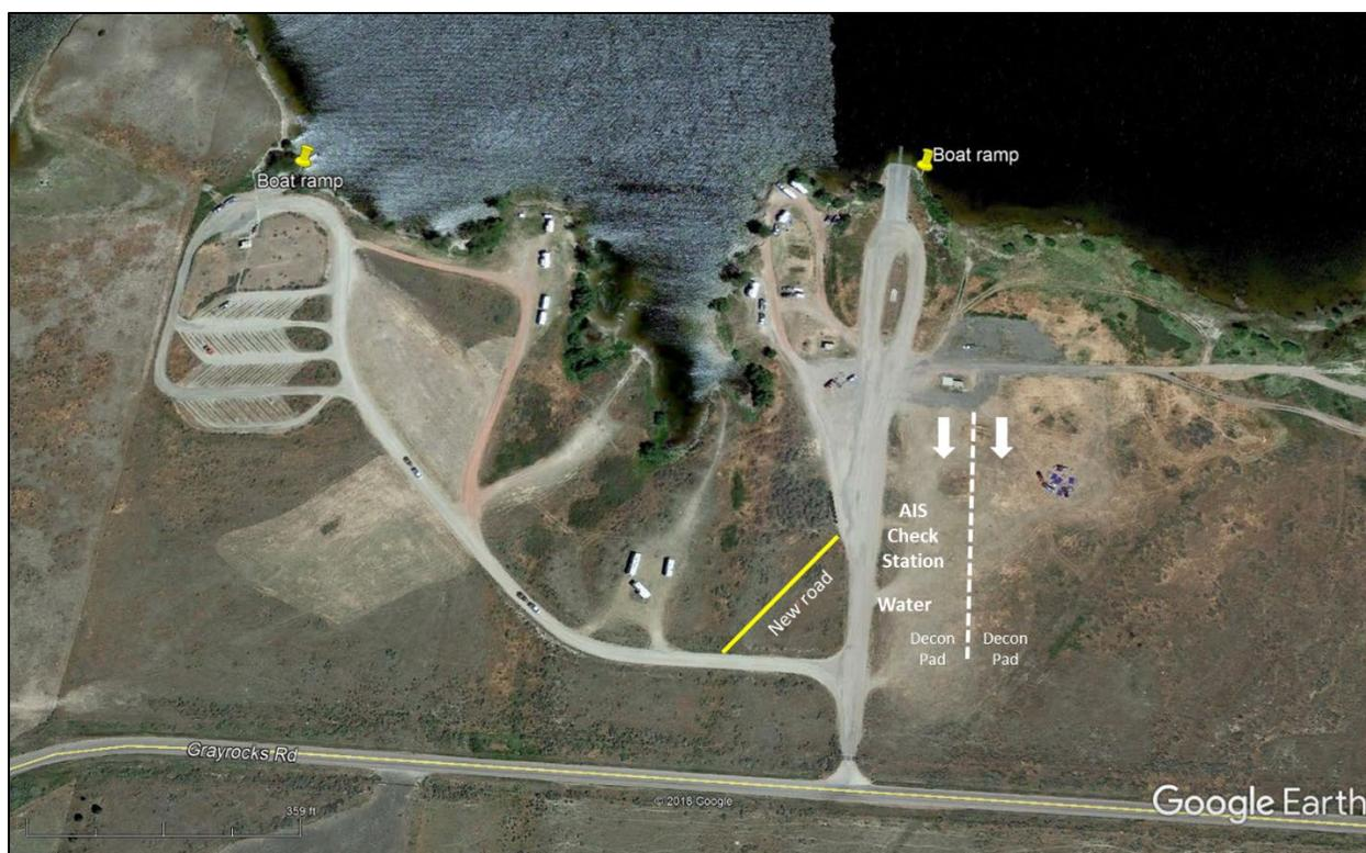
FIGURE 4. Two western-most boat ramps at Grayrocks Reservoir and layout of the AIS check station, decontamination pads, and water storage area during Long-term Suspect Status. White arrows show direction for two decontamination pads and yellow line shows location of a new road.
