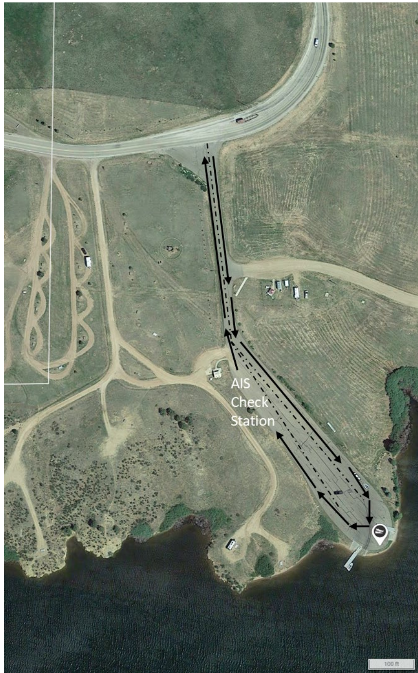
FIGURE 5. Overview map of Granite Reservoir parking lot and boat ramp. Temporary AIS check station location shown in white text and new one-way traffic flow shown with black arrows.
