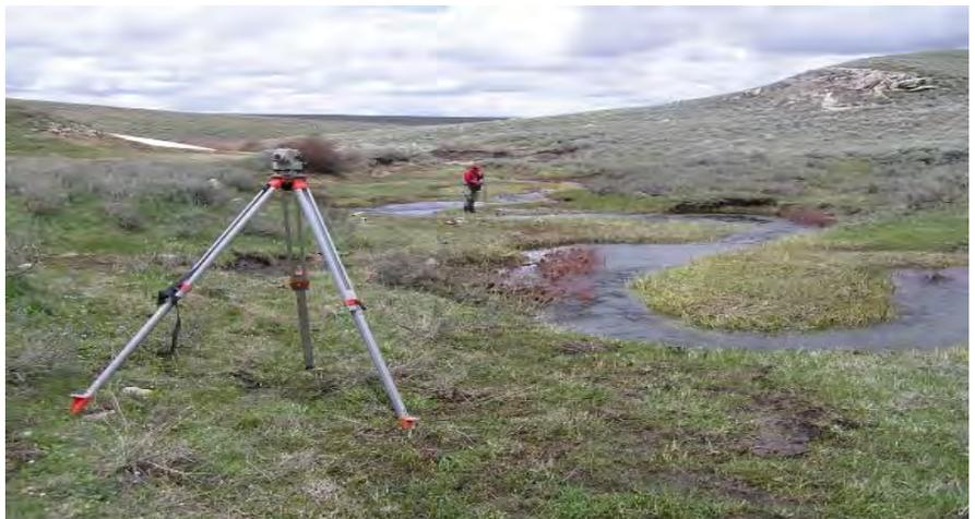
Figure 4. Instream flow studies were conducted on four streams flowing through the WGFD Grizzly Wildlife Habitat Management Area including Little Muddy Creek shown here. Field studies require collecting flow data at several different flow levels.
