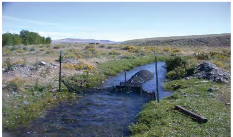
Figure 10. Sampling net in the Ashworth No. 3 Ditch to evaluate Yellowstone cutthroat trout entrainment.
