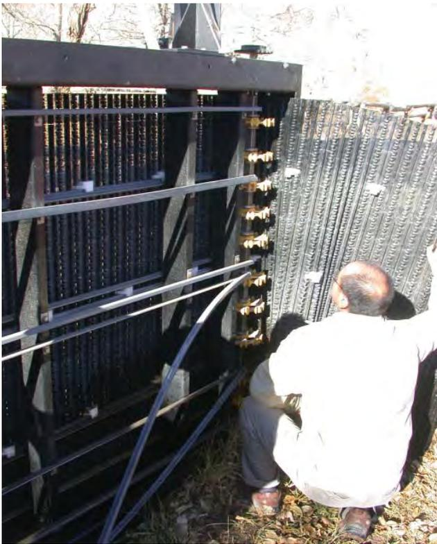
Figure 11. A Hydrolox engineer evaluates the horizontal traveling screen for potential modifications.
