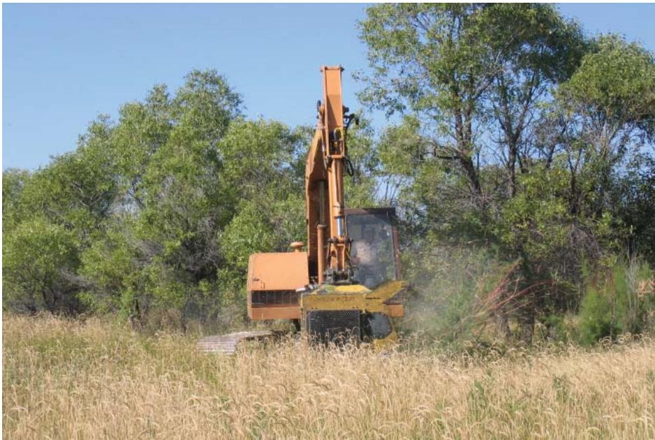
Figure 1. Mechanical removal of saltcedar on Beaver Creek.
