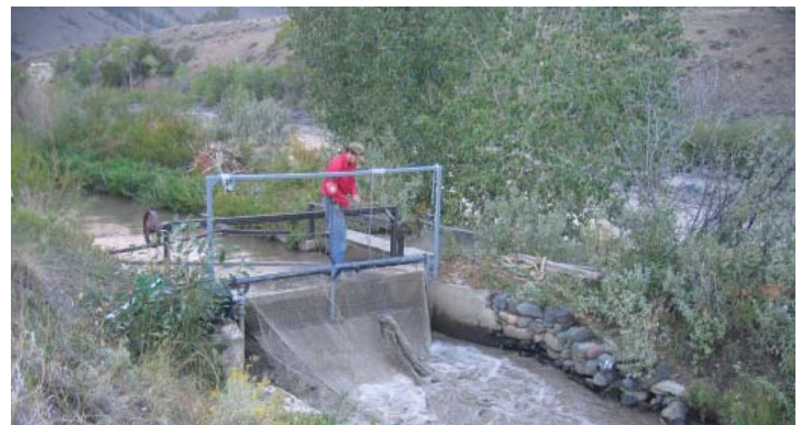
Figure 13. Structure and associated netting for evaluating fish loss down the North Fork Canal.
