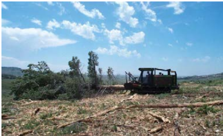
Figure 1. GyroTrac equipment used to mechanically treat aspen stands.
