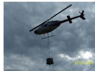
Helicopters with a fish stocking tank are used to stock remote lakes.
