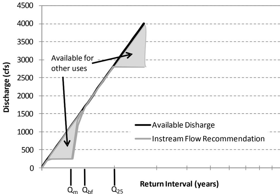
FIGURE B-2. Generalized dynamic hydrograph indicating recommended instream flow for fishery maintenance.  $Q_m$  is substrate mobilization flow,  $Q_{bf}$  is bankfull flow, and  $Q_{25}$  is the discharge with a 25-year return interval.
