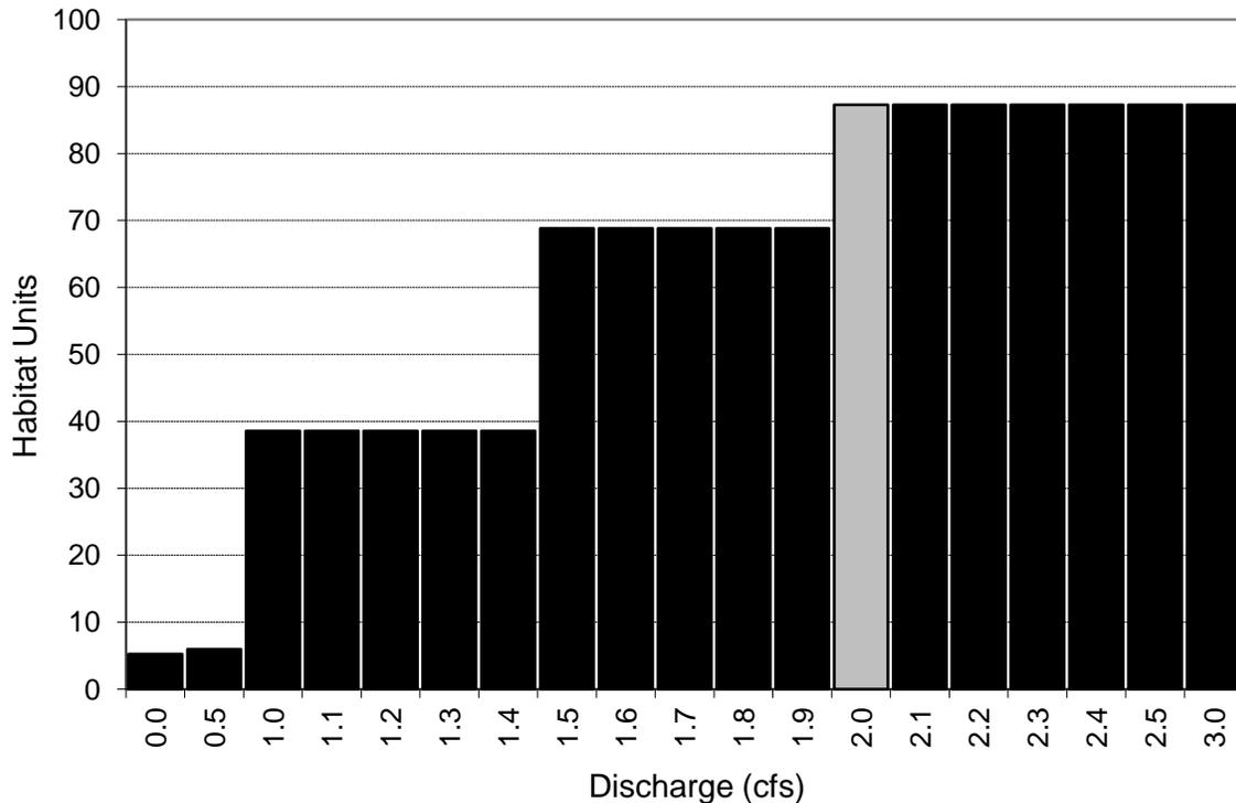
FIGURE 9. Habitat Quality Index vs. discharge in the Trout Creek instream flow segment. X-axis values are not to scale; the values were chosen to indicate where changes in Habitat Units occur. The recommended flow is indicated by the light shaded bar.
