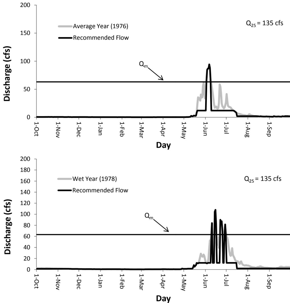
FIGURE B-3. Channel maintenance flow recommendations and hydrographs for the Trout Creek instream flow segment in an average (1976) and a wet (1978) water year.
