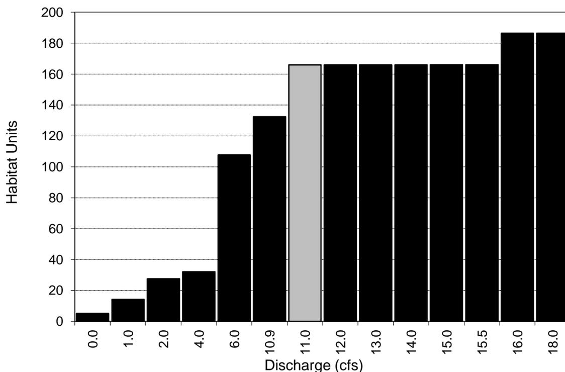
FIGURE 9. Habitat Quality Index vs. discharge in the Cedar Creek instream flow segment. X-axis values are not to scale; the values were chosen to indicate where changes in Habitat Units occur. The recommended flow is indicated by the light shaded bar.
