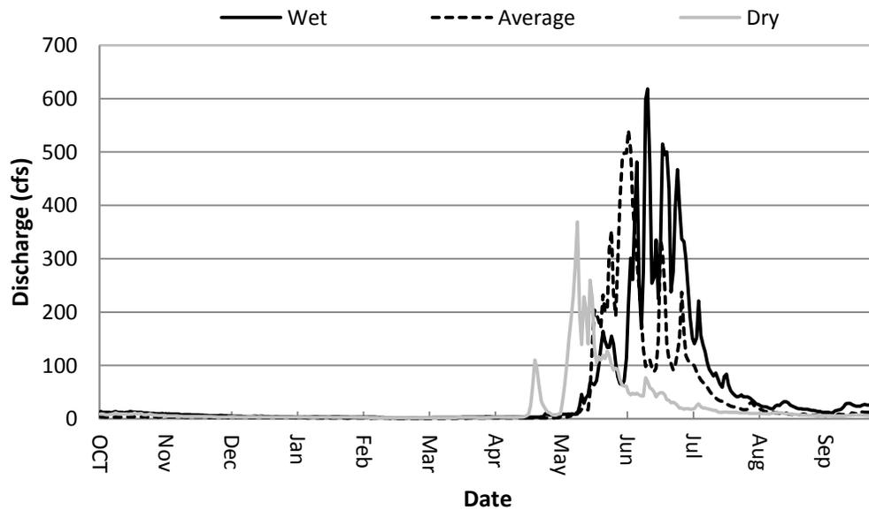
FIGURE 5. Hydrographs for representative wet (1978), average (1976), and dry (1994) water years from the Shell Creek USGS stream gage station (06278300). Representative years were randomly selected from within each of three flow exceedance classes (wet 0–10%, average 30–70%, and dry 90–100%).
