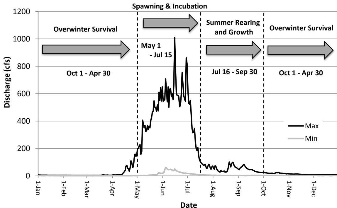
FIGURE 6. Lowest and highest daily historical discharge values in the reference gage for this study with critical time periods for YCT distinguished. Data is from the reference gage for this study, USGS gage 06278300 on Shell Creek above Shell Reservoir (1956-present).
