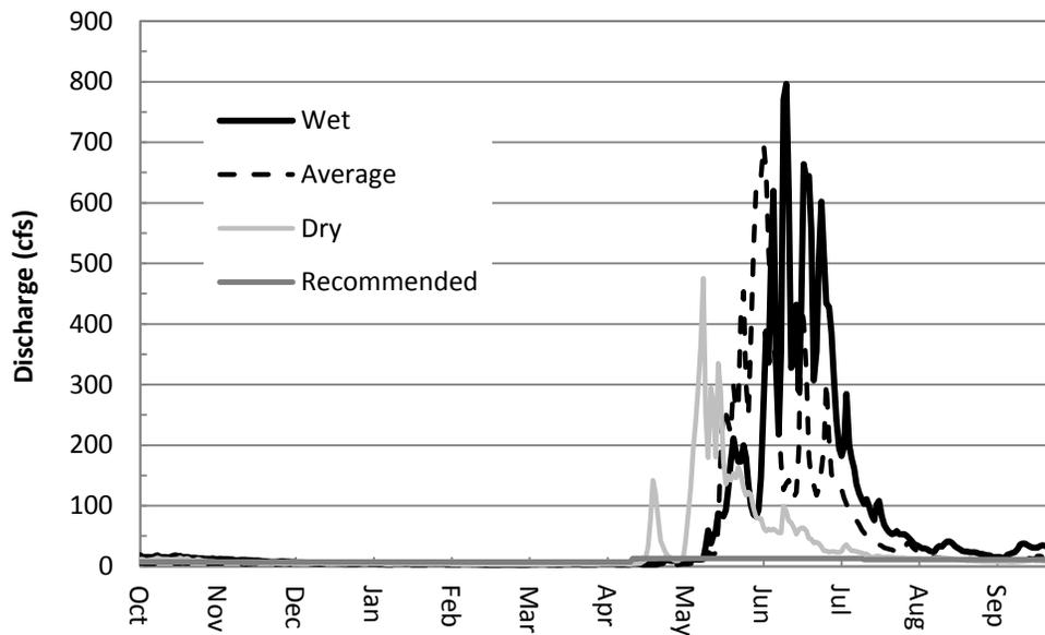
FIGURE 10. Recommended instream flow water right in the proposed segment (when naturally available) relative to wet, dry, and average flow years.
