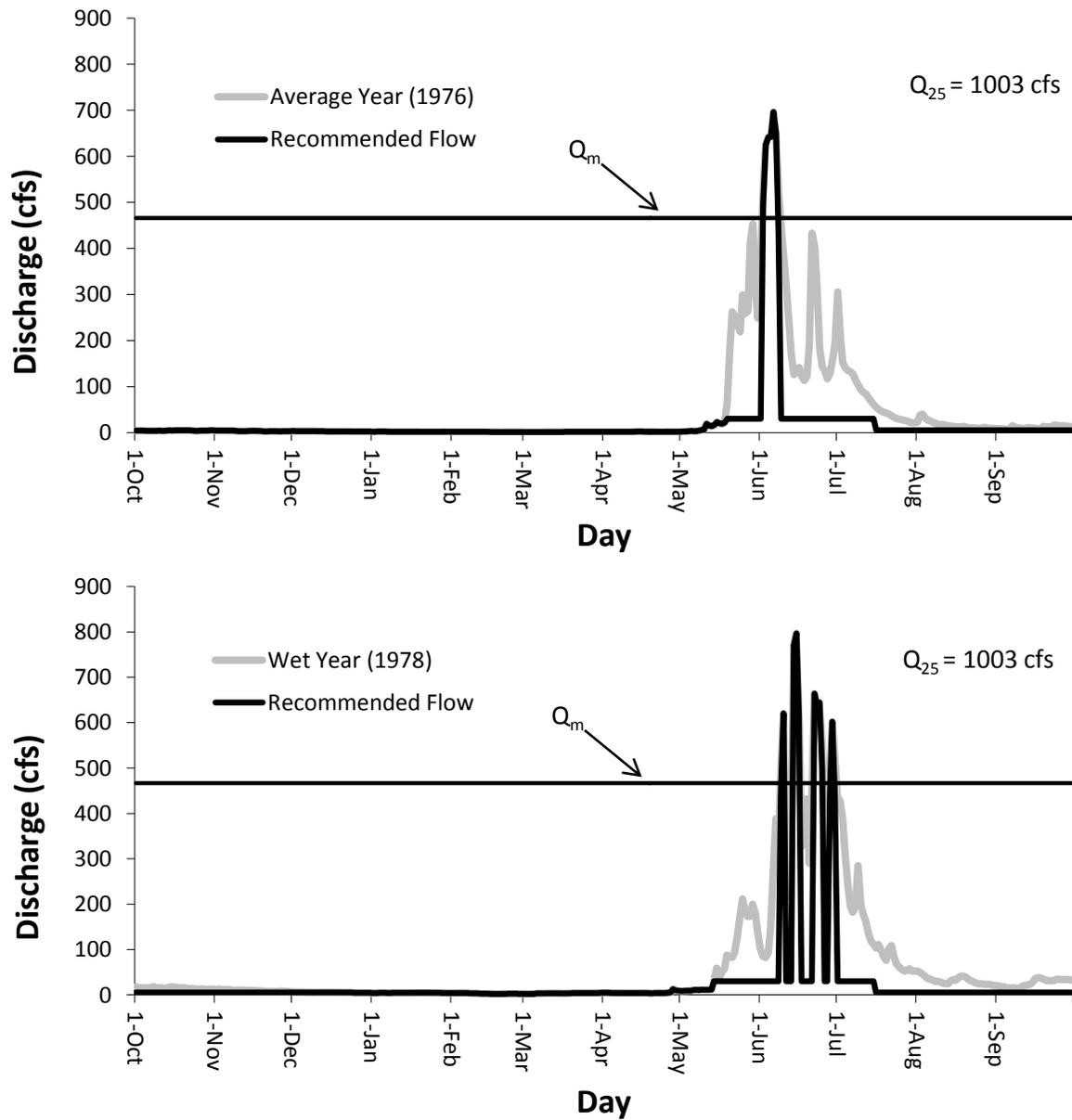
FIGURE B-3. Channel maintenance flow recommendations and hydrographs for the Cedar Creek instream flow segment in an average (1976) and a wet (1978) water year.
