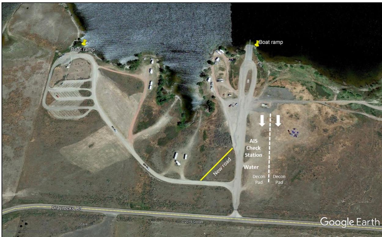
FIGURE 4. Two western-most boat ramps at Grayrocks Reservoir and layout of the AIS check station, decontamination pads, and water storage area during Long-term Suspect Status. White arrows show direction for two decontamination pads and yellow line shows location of a new road.
