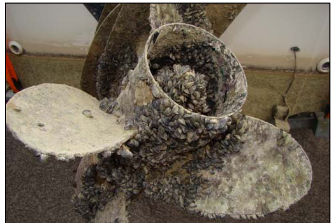
The prop and exhaust of this outboard motor are covered with Quagga mussels after the boat was docked in Lake Mead for 6 months.
