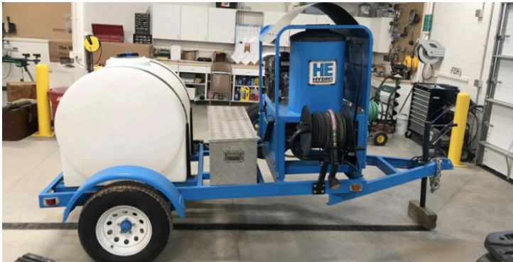
AIS decontamination unit - the pressure washer with very hot water to clean invasive species off boats.
