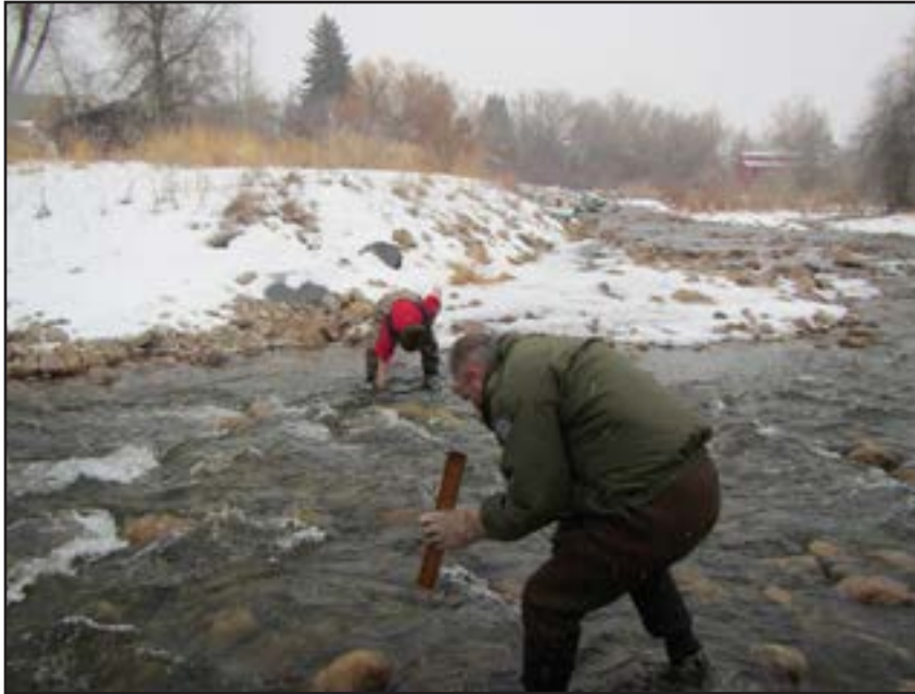
Figure 74. Collecting pebble counts to document existing substrate conditions and to compare to future conditions.
