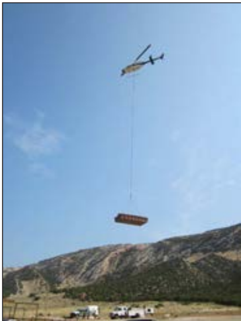
Figure 32. A Type III helicopter slings a guzzler to its new location.
