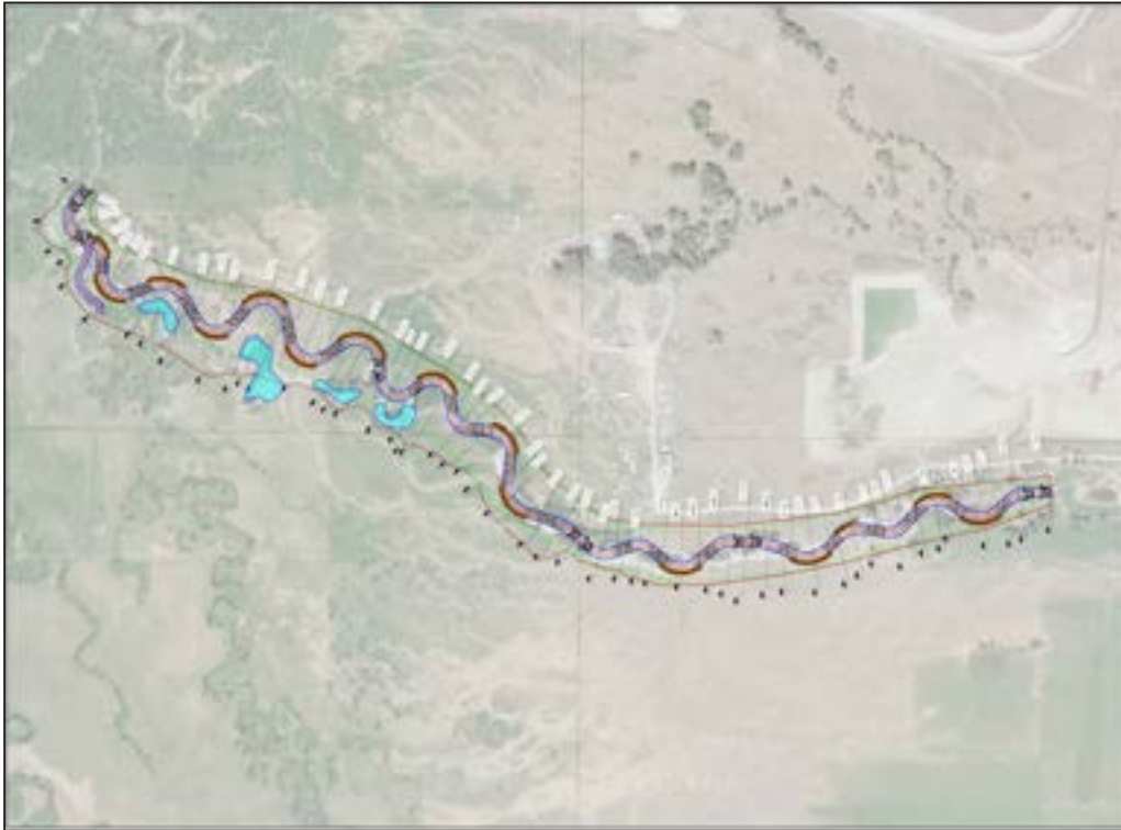
Figure 96. Swift Creek design illustrating extensive channel realignment, bank treatments and establishment of appropriate pool and riffle spacing.
