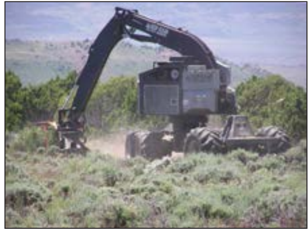
Figure 77. Masticating junipers to increase grass, forb and shrub production for mule deer and sage grouse. Photo courtesy of Little Snake River Conservation District.
