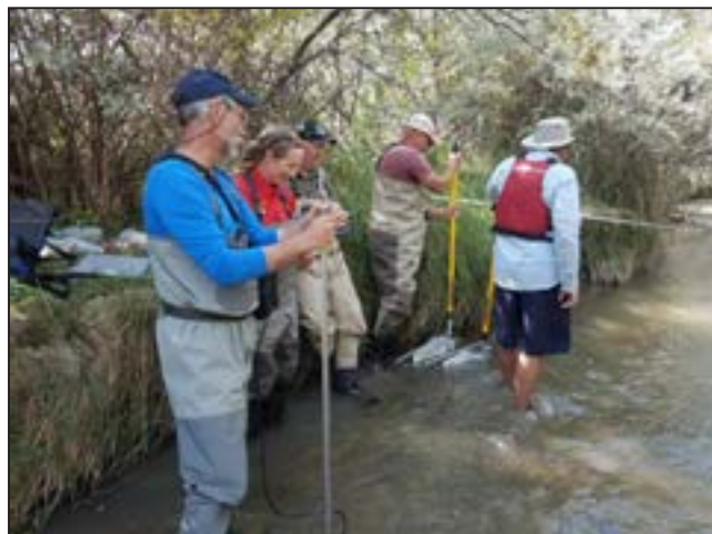
Figure 43. WGFD and DEQ staff collecting suspended sediment and bedload data from Idaho Creek, a tributary to the Lower Shoshone River.
