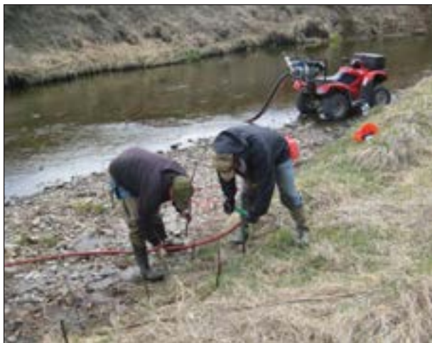
Figure 163. ATV mounted water pump and stinger attachment for planting cuttings.
