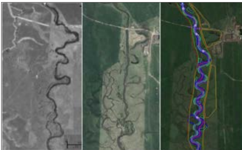
Figure 74. Flat Creek stream pattern over time: 1945 (left), 2015 (center), proposed (right).
