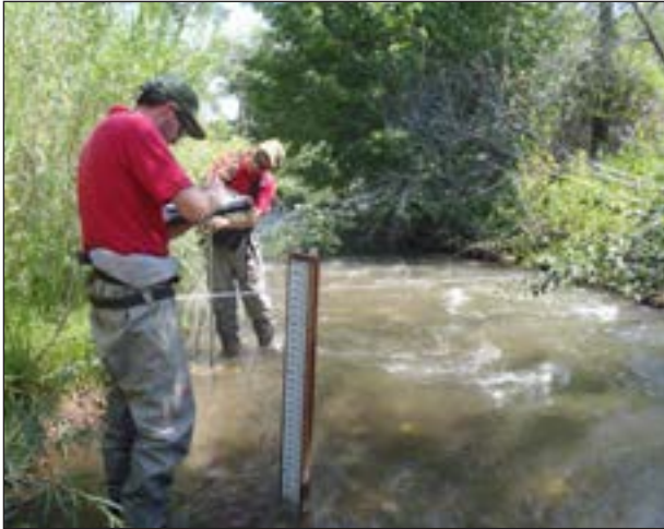
Figure 7. Trout Creek staff gage and habitat personnel measuring flow.
