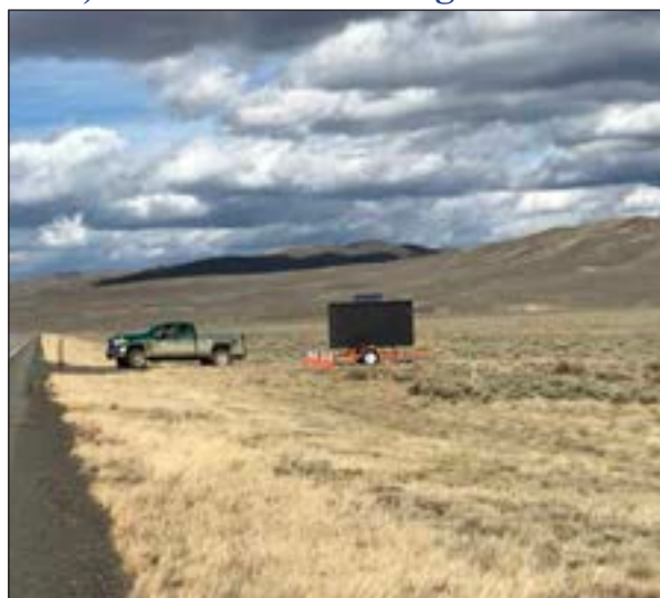
Figure 121. Dynamic messaging signs deployed by WGFD and WYDOT in big game high use areas.
