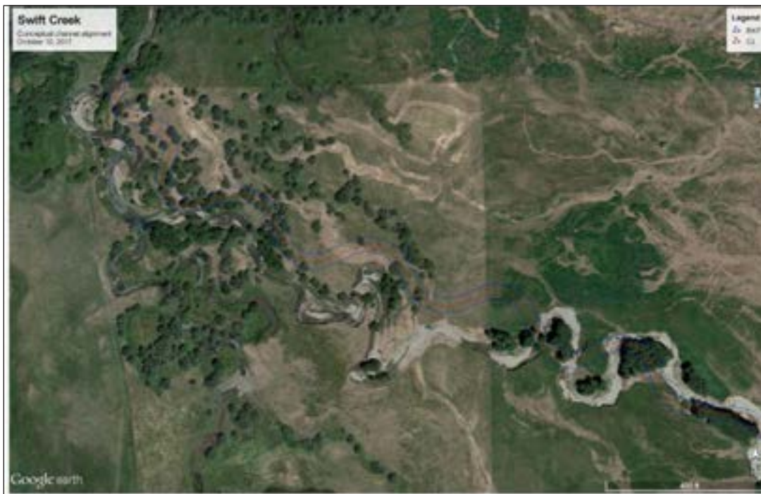
Figure 70. Design showing Swift Creek channel realignment (red line).
